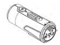
Check that the camera power is turned OFF. Insert a MicroSD card (with the printed side up) into the MicroSD Card Slot with enough finger pressure to keep the edge of the card flush with the card slot opening.
